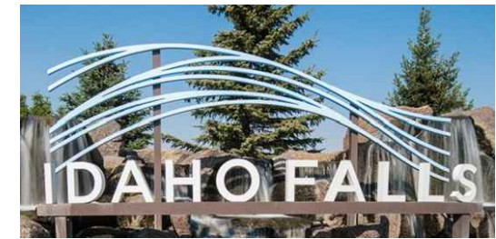
SILVER ALUMINUM "WAVES" EXAMPLE: AVERAGE 2" SILVER ALUMINUM "WAVES" ON TOP AND IN FRONT OF MONUMENT SIGN ATTACHED WITH ALUMINUM SUPPORT RODS
