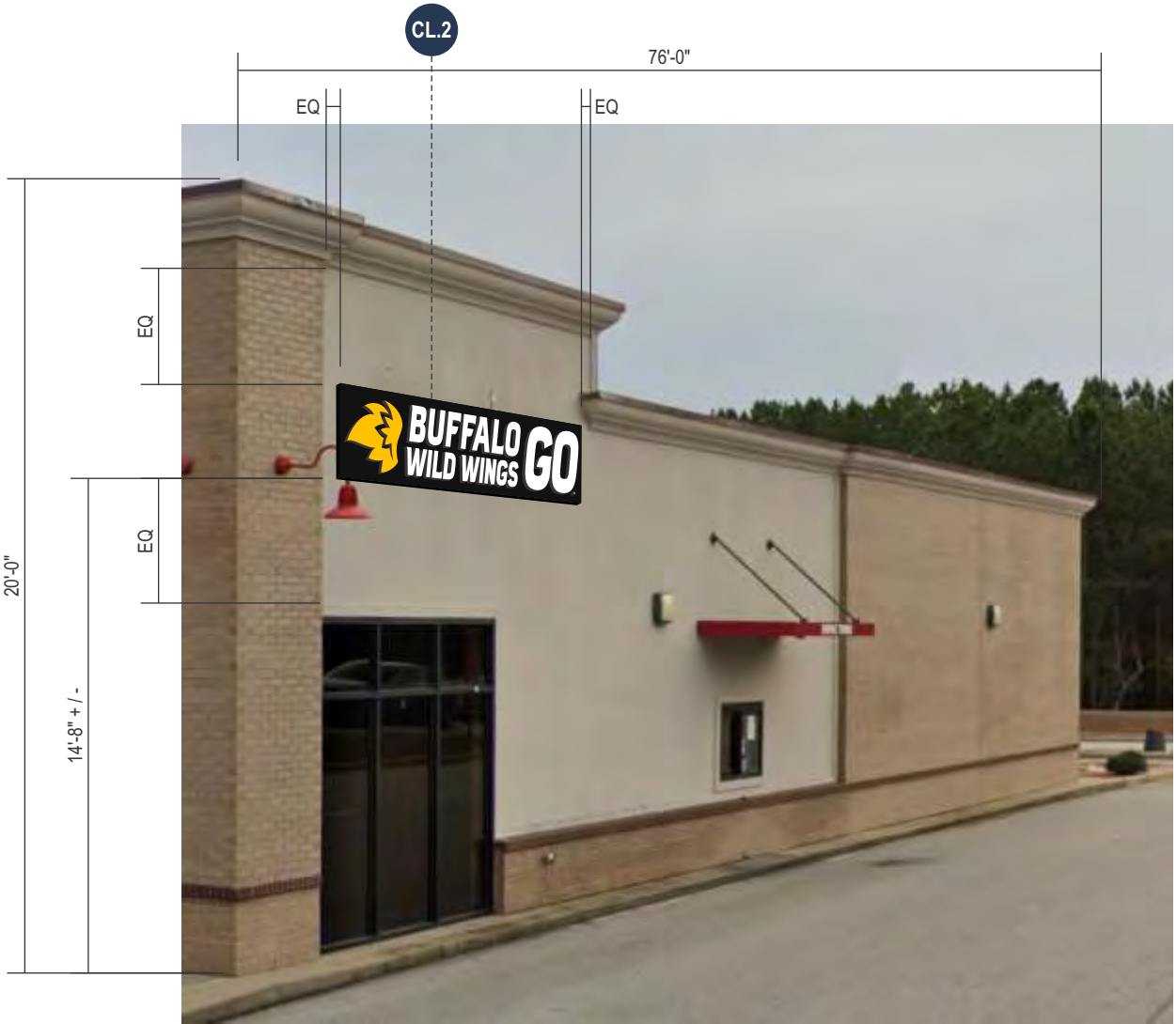
WEST ELEVATION - PROPOSED SIGNAGE SCALE: APPROX. 3/16" = 1'-0" NOTE: PROPOSED REPRESENTATION IS NOT TO EXACT SCALE AND PROPORTIONS MAY VARY FROM ACTUAL SIZING.
