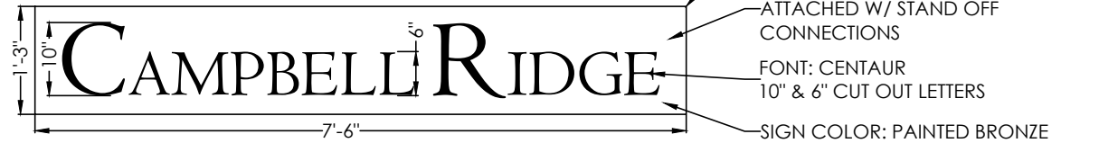
1 SIGN PANEL DETAIL S-1.4 SCALE: 1/2"=1'
