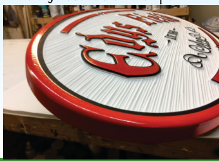
HDU Sign Face w/ Grain Example
