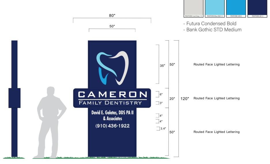
Quantity: 1 Monument Sign - 80" Wide x 120" Tall x 12" Deep Overall Size; Heavy Gauge Extruded Aluminum Cabinet, Welded and Sealed LED Lit Pylon Sign; Cut-Thru Tooth Logo - Top Panel; Cut-Thru Business Name Lettering -Center Panel; Cut Through Lettering - Lower Panel; Sign Painted 2 Colors; Decorated With 3M Translucent Vinyl, 3M IJ40C Vinyl & Day/Night Perf; Single Steel Pole Mounted
