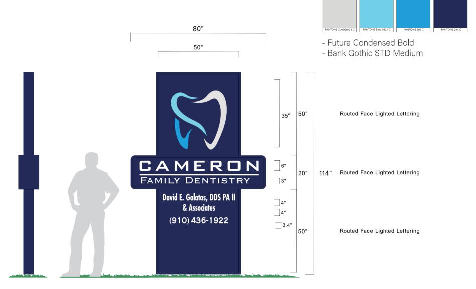
Quantity: 1 Monument Sign - 80" Wide x 114 " Tall x 12" Deep Overall Size; Heavy Gauge Extruded Aluminum Cabinet, Welded and Sealed LED Lit Pylon Sign; Cut-Thru Tooth Logo - Top Panel; Cut-Thru Business Name Lettering -Center Panel; Cut Through Lettering - Lower Panel; Sign Painted 2 Colors; Decorated With 3M Translucent Vinyl, 3M IJ40C Vinyl & Day/Night Perf; Single Steel Pole Mounted
