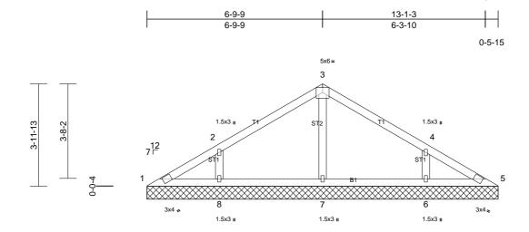
Loading Spacing 2-0-0 CSI **DEFL** I/defI L/d **PLATES** GRIP (psf) (loc) TCLL (roof) 20.0 Plate Grip DOL 1.15 TC 999 244/190 0.20 Vert(LL) n/a n/a MT20 BC **TCDL** 10.0 Lumber DOL 1.15 0.12 Vert(TL) n/a n/a 999 **BCLL** 0.0 Rep Stress Incr YES WB 0.07 Horiz(TL) 0.00 5 n/a n/a **BCDL** 10.0 IRC2015/TPI2014 Matrix-MSH Weight: 50 lb FT = 20% Code
