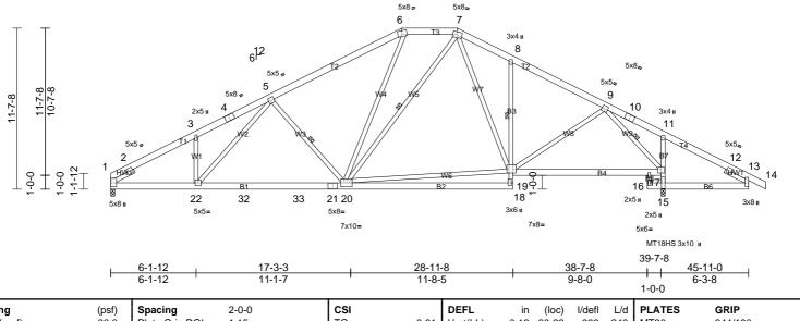
Loading TCLL (roof) 20.0 Plate Grip DOL 1.15 TC 0.61 Vert(LL) -0.19 20-22 >999 240 MT20 244/190 BC **TCDL** 10.0 Lumber DOL 1.15 0.84 Vert(CT) -0.3420-22 >999 180 MT18HS 244/190 **BCLL** 0.0 Rep Stress Incr YES WB 0.57 Horz(CT) 0.05 15 n/a n/a **BCDL** 10.0 IRC2015/TPI2014 Matrix-MSH Weight: 376 lb FT = 20% Code
