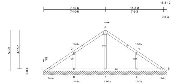
Loading Spacing 2-0-0 CSI **DEFL** I/defI L/d **PLATES** GRIP (psf) (loc) TCLL (roof) 20.0 Plate Grip DOL 1.15 TC 999 244/190 0.23 Vert(LL) n/a n/a MT20 BC **TCDL** 10.0 Lumber DOL 1.15 0.12 Vert(TL) n/a n/a 999 **BCLL** 0.0 Rep Stress Incr YES WB 0.13 Horiz(TL) 0.00 5 n/a n/a **BCDL** 10.0 IRC2015/TPI2014 Matrix-MSH Weight: 63 lb FT = 20% Code
