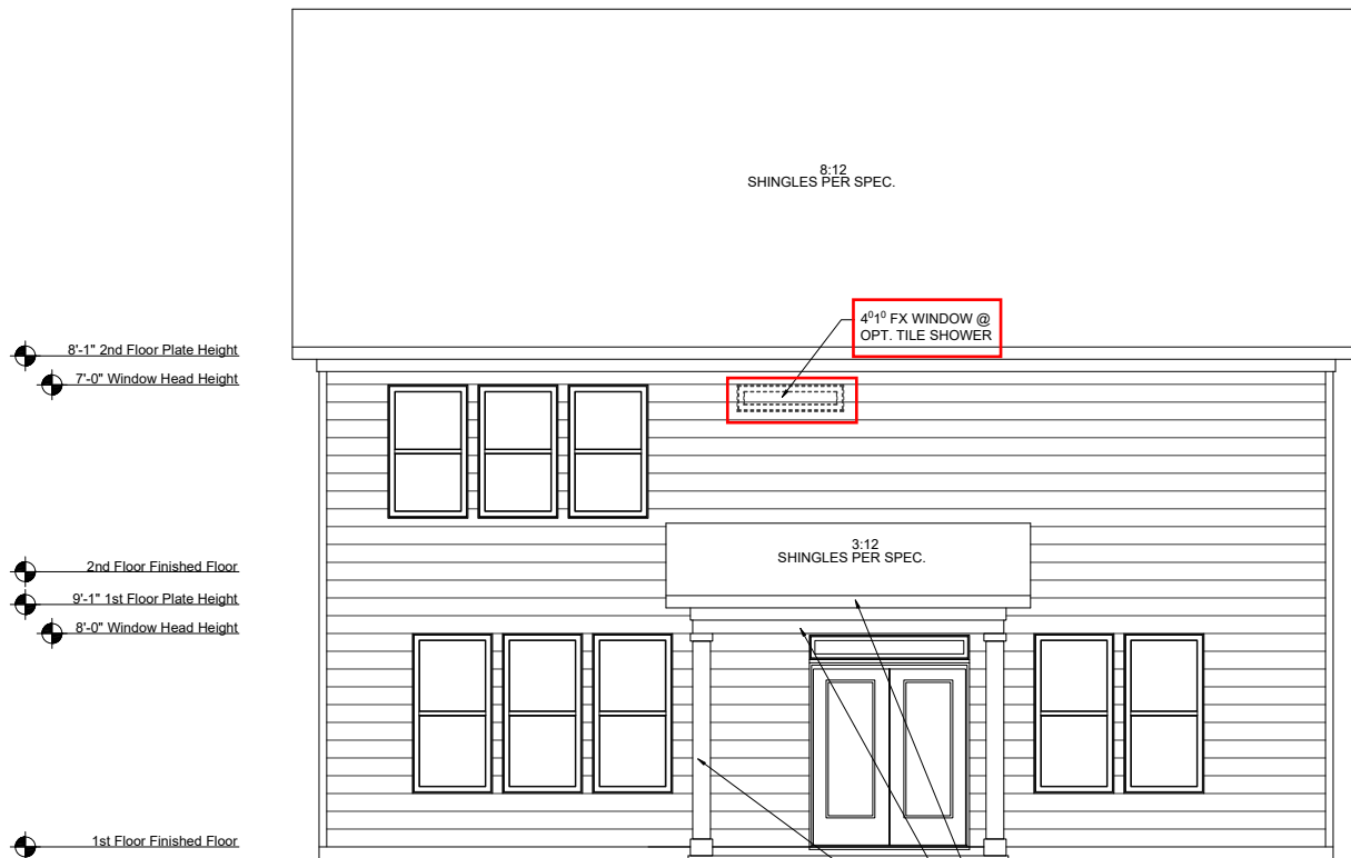
COVERED PORCH REAR ELEVATION SCALE: 1/8"=1'-0" (11"x17" SHEET SIZE) SCALE: 1/4"=1'-0" (22"x34" SHEET SIZE)
