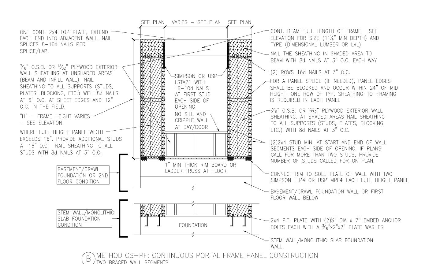
WINDOW OR DOOR REINFORCEMENT IN ENGINEERED SHEAR WALL JONLY REQUIRED WHERE SPECIFIED ON PLANS
