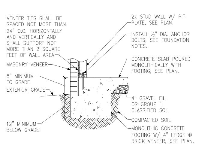
FOUNDATION SECTION EXTERIOR WALL @ MASONRY VENEER
