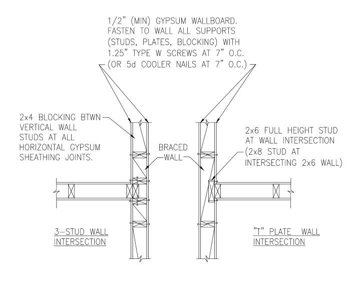
BRACED WALL INTERSECTIONS MAY BE FRAMED USING EITHER THE 3-STUD OR THE T-PLATE METHOD.
