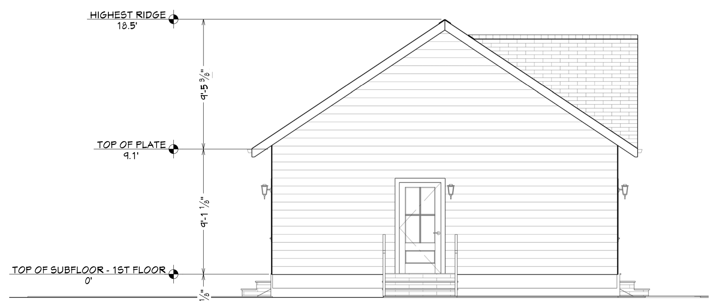
E2 EXTERIOR ELEVATION LEFT 1/4 IN = 1 FT
