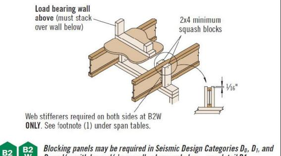
IRC 502.7 requires lateral restraint (blocking) at all intermediate supports in Seismic Design Categories  $D_0$ ,  $D_1$ , and  $D_2$  to strengthen the floor diaphragm
