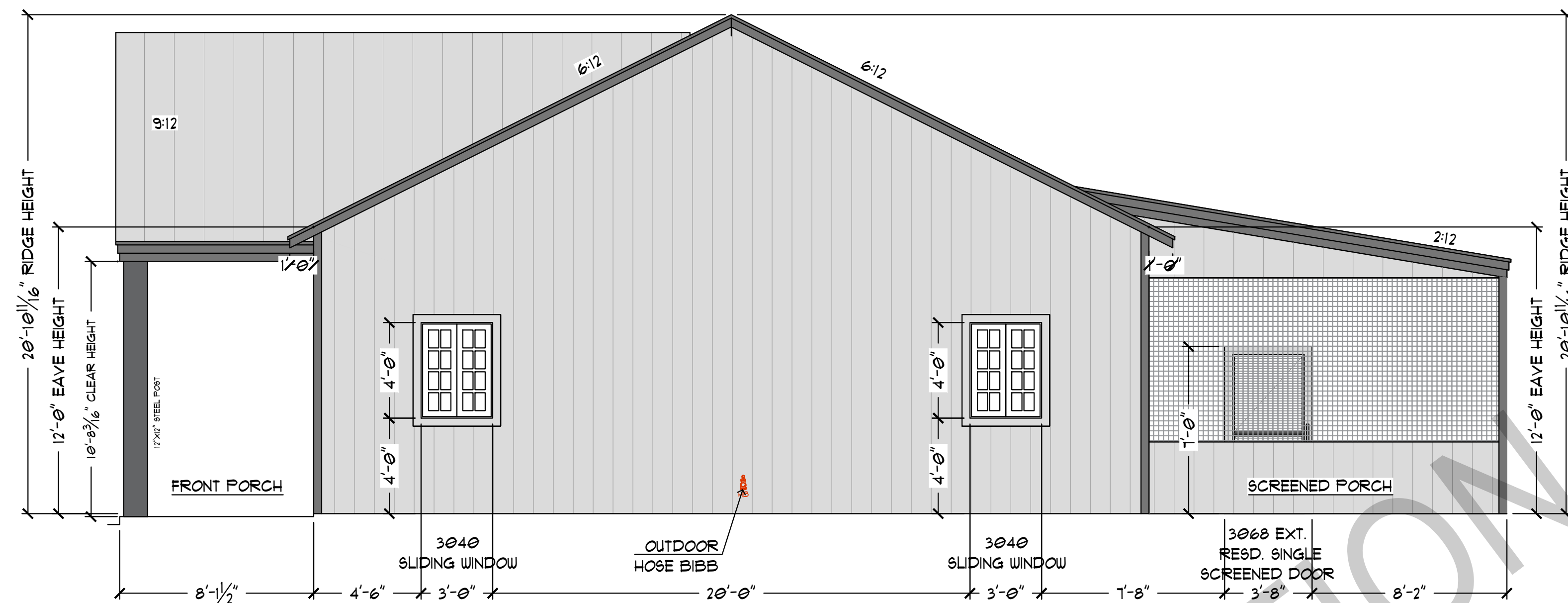
RIGHT SIDE ELEVATION SCALE: 1/4" = 1'-0"
