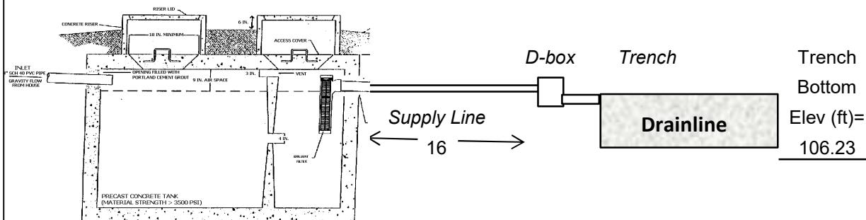
\*Outlet depth of septic tank is dependant upon the depth of the plumbing stub out from the home.
