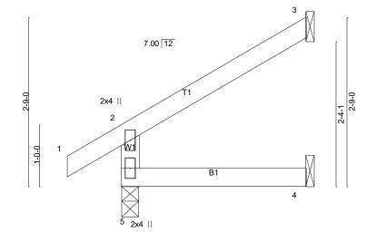
LOADING (psf) SPACING-2-0-0 CSI. DEFL. in (loc) I/defl L/d 20.0 TCLL (roof) Plate Grip DOL 1.15 TC 0.17 Vert(LL) -0.00 4-5 >999 240 Snow (Pf) 20.0 Lumber DOL ВС 0.10 Vert(CT) -0.01 >999 180 1.15 4-5 TCDL 10.0 Rep Stress Incr YES WB 0.00 Horz(CT) -0.01 3 n/a n/a BCLL 0.0 Code IRC2021/TPI2014 Matrix-MR BCDI 10.0
