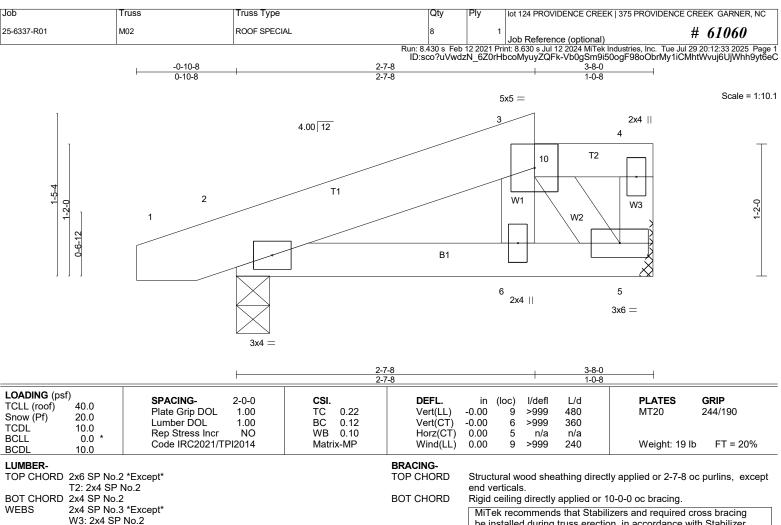
be installed during truss erection, in accordance with Stabilizer Installation guide.
