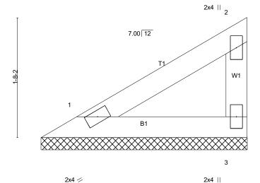
LOADING (psf) DEFL. SPACING-**PLATES** GRIP 2-0-0 CSI in (loc) I/defl I/d 20.0 TCLL (roof) Plate Grip DOL 1.15 TC 0.12 Vert(LL) n/a n/a 999 MT20 244/190 Snow (Pf) 20.0 Lumber DOL ВС 0.09 Vert(CT) 999 1.15 n/a n/a TCDL 10.0 Rep Stress Incr YES WB 0.00 Horz(CT) 0.00 n/a n/a BCLL 0.0 Code IRC2021/TPI2014 Matrix-P Weight: 10 lb FT = 20% BCDI 10.0
