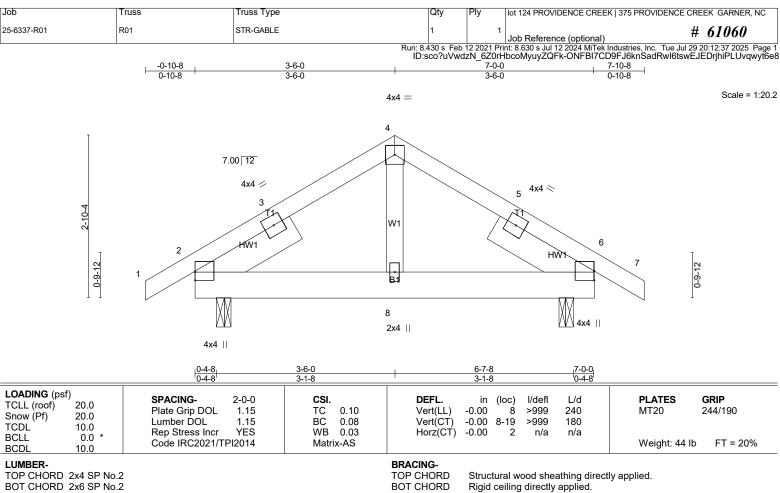
MiTek recommends that Stabilizers and required cross bracing be installed during truss erection, in accordance with Stabilizer Installation guide
