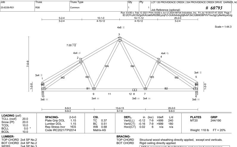
MiTek recommends that Stabilizers and required cross bracing be installed during truss erection, in accordance with Stabilizer Installation guide
