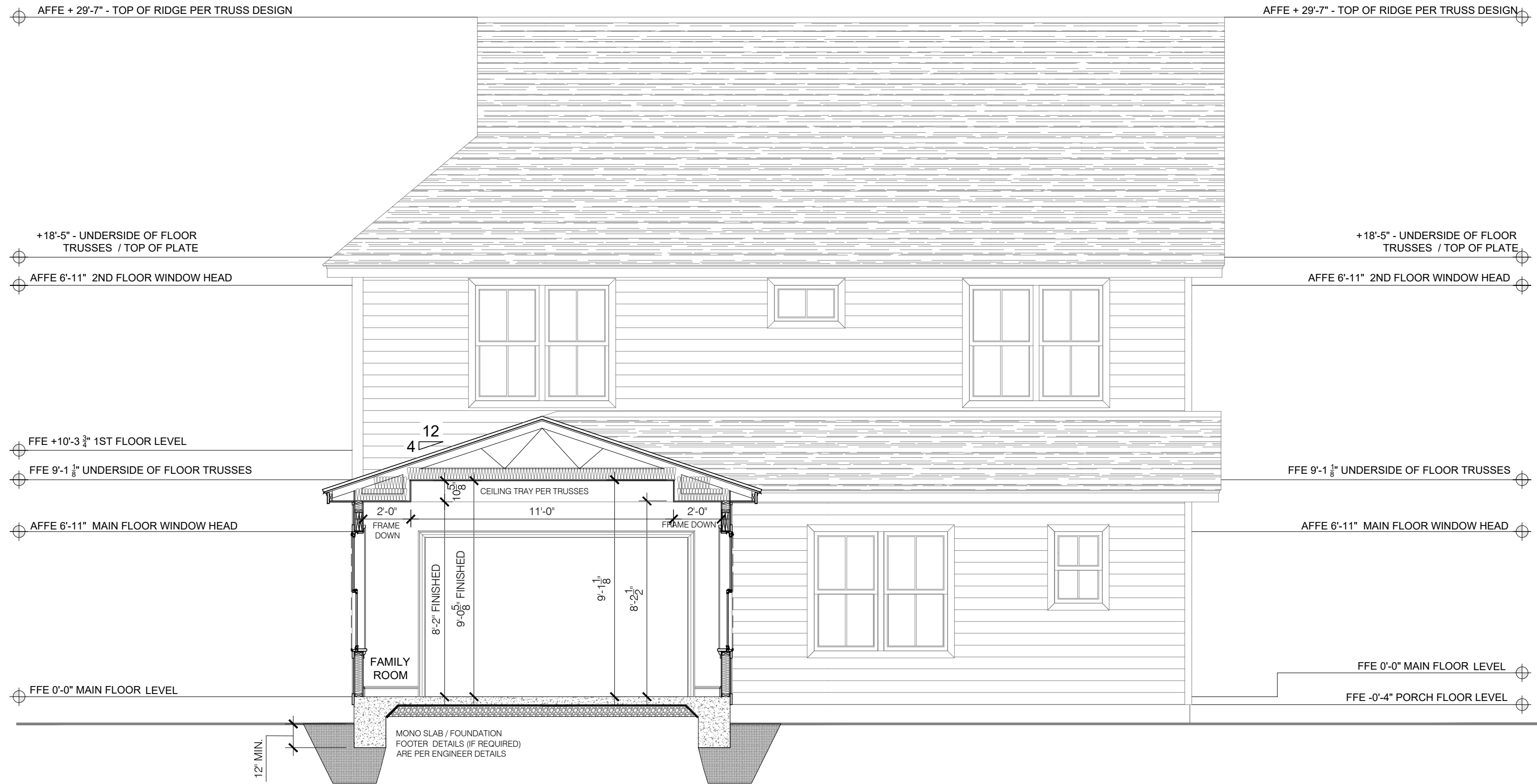
BUILDING SECTION (SEE STANDARD FLOOR PLAN) - 2 SCALE: 1/4" = 1'-0"
