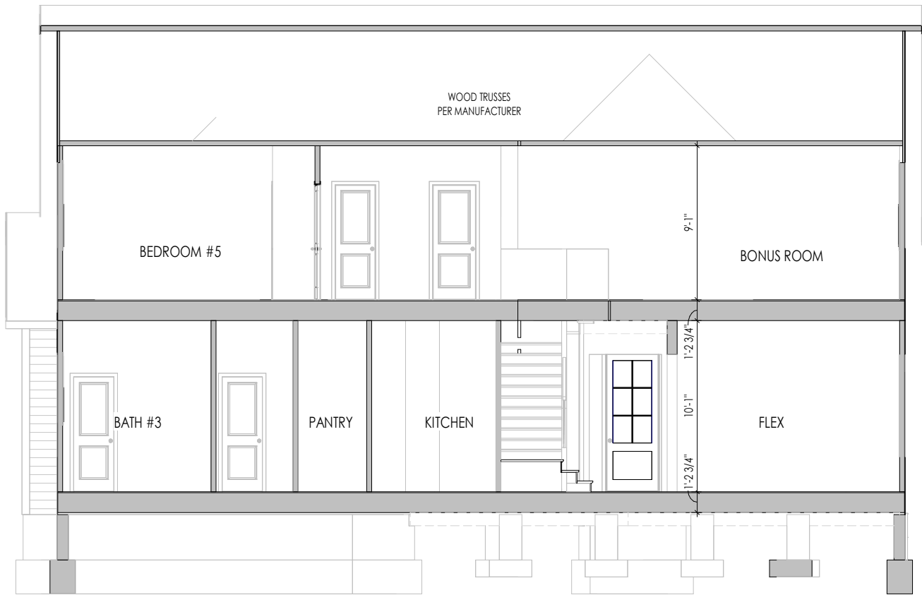
A 5.01 BUILDING SECTION THRU FAMILY ROOM 1/8" = 1'-0"
