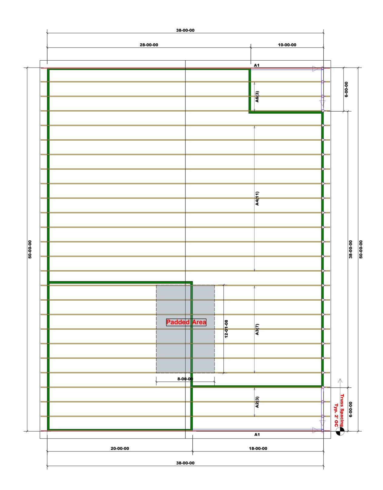
= Indicates Left End of Truss (Reference Engineered Truss Drawing) Do NOT Erect Truss Backwards
