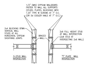
BE FRAMED USING EITHER THE 3-STUD OR THE T-PLATE METHOD.
