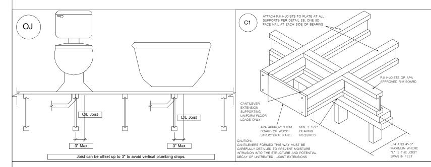
PLUMBING DROPS NOTED ARE IN APPROXIMATE LOCATIONS PER PLAN. BUILDER MUST VERY LOCATIONS BEFORE SETTING JOISTS.
