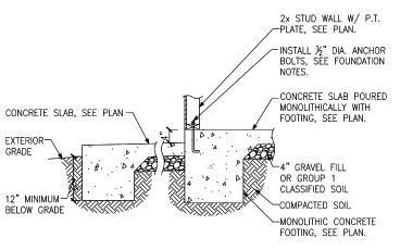
C FOUNDATION SECTION EXTERIOR WALL AT PORCH
