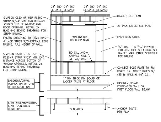
C WINDOW OR DOOR REINFORCEMENT IN ENGINEERED SHEAR WALL ONLY REQUIRED WHERE SPECIFIED ON PLANS
