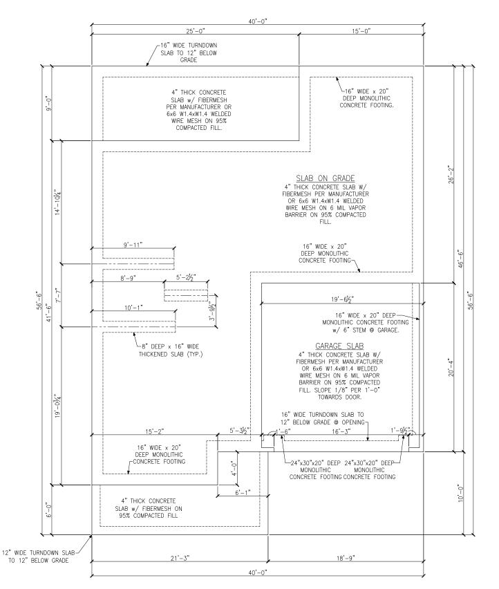
MONOLITHIC SLAB FOUNDATION PLAN ELEVATION E
