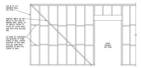
NOTE: BLOCKING AND SIMPSON STRAPS ARE NOT REQUIRED IF WALL IS SHEATHED ON ONE FACE WITH GYPSUM WALL BOARD
