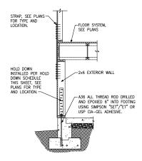
(C)HOLD DOWN AT STEMWALL SLAB
