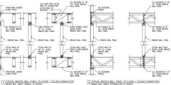
B TYPICAL BRACED WALL PANEL TO FLOOR / CEILING CONNECTION BRACED WALL PANELS PERPENDICULAR TO TRUSSES
