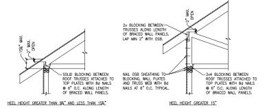
(D) TYPICAL EXTERIOR CORNER WALL FRAMING
