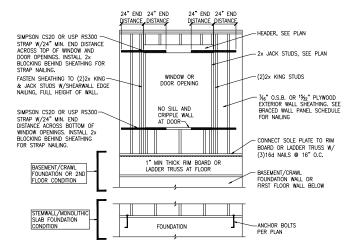
© WINDOW OR DOOR REINFORCEMENT IN ENGINEERED SHEAR WALL ONLY REQUIRED WHERE SPECIFED ON PLANS
