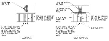
E BUILT-UP STUD DETAIL SUPPORTING BEAM
