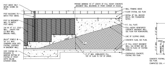
A FOUNDATION ELEVATION STEPPED SIDEWALL
