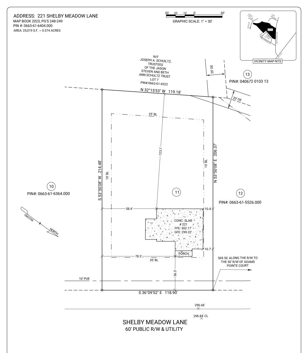
**LEGEND Public Drainage Easement** PDE N/F Now or Formerly FΡ Electric Pedestal Drainage Easement DE BL**Building Line** PΒ Phone Box Parcel Identification PIN Finished Floor Elevation TBOX Telephone Box FFE Number Cable TV **GFE** Garage Floor Elevation CATV HGT Height PROP Proposed CO Clean Out
