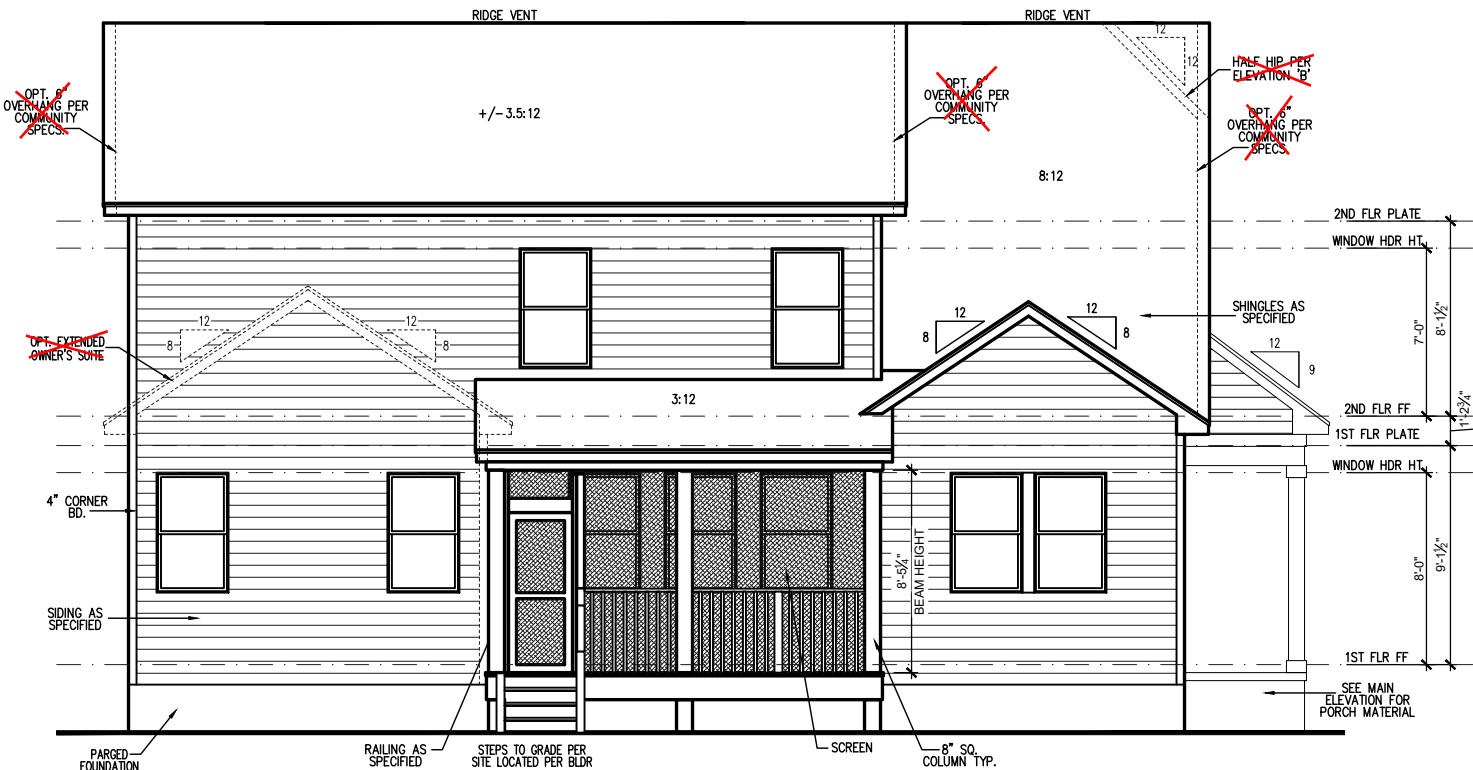
BEDROOM 4 W/ SCR. PORCH REAR ELEVATION SCALE: 1/8"=1'-0" ON 11x17, 1/4"=1'-0" ON 22x34
