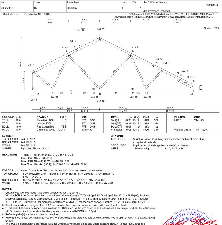
7) This truss is designed in accordance with the 2018 International Residential Code sections R502.11.1 and R802.10.2 and referenced standard ANSI/TPI 1.
