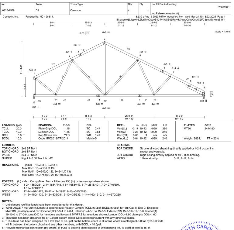
6) This truss is designed in accordance with the 2018 International Residential Code sections R502.11.1 and R802.10.2 and referenced standard ANSI/TPI 1.
