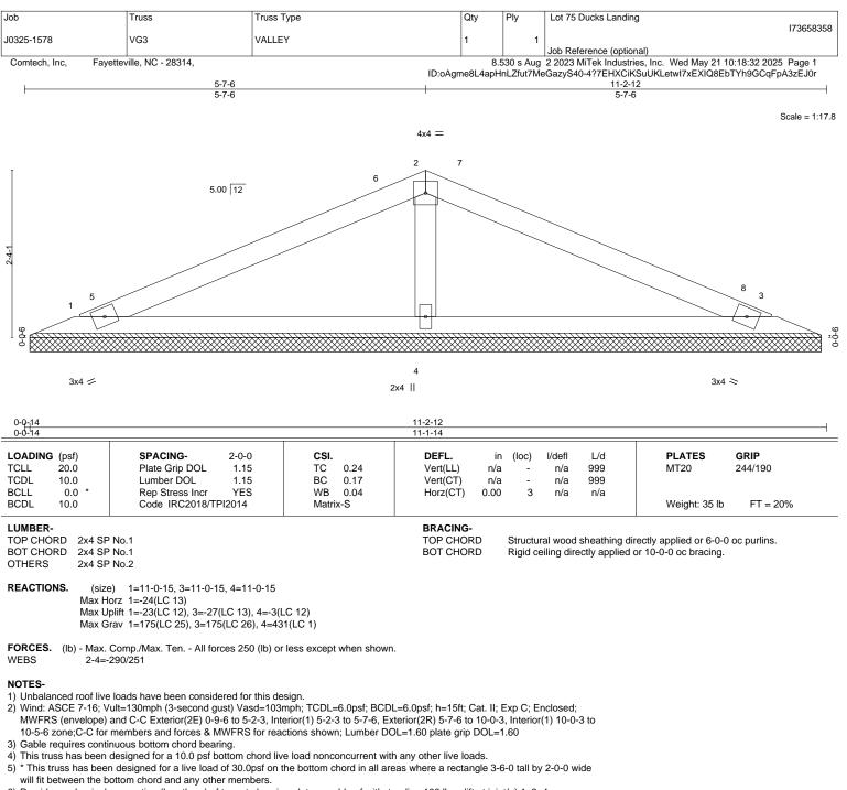
6) Provide mechanical connection (by others) of truss to bearing plate capable of withstanding 100 lb uplift at joint(s) 1, 3, 4.
