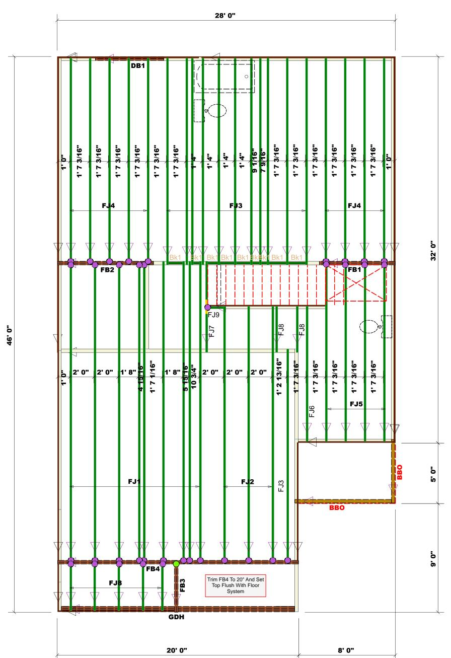
Plumbing Drop Notes 1. Plumbing drop locations shown are NOT exact. 2. Contractor to verify ALL plumbing drop locations prior to setting Floor Trusses. 3. Adjust spacing as needed not to exceed 19.2
