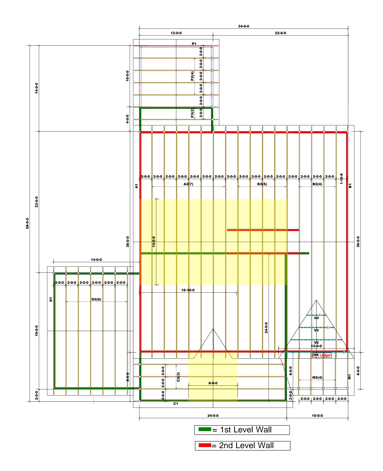
A = Indicates Left End of Truss (Reference Engineered Truss Drawing) Do NOT Erect Truss Backwards
