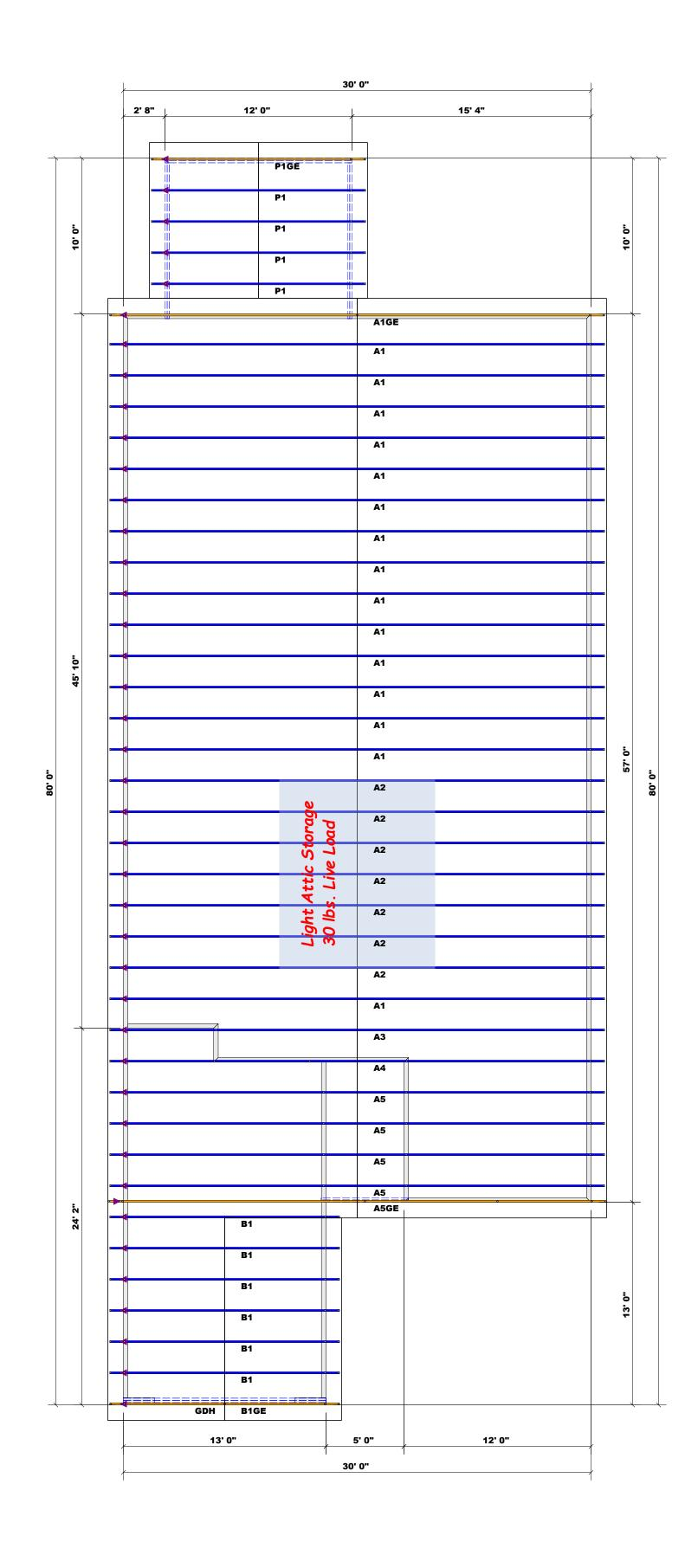
▲ = Denotes Left End of Truss (Reference Engineered Truss Drawing) Do Not Erect Trusses Backwards
