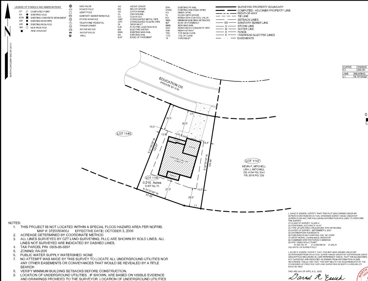
D. LOCATION OF UNDERGROUND UTILITIES, IF SHOWN, ARE BASED ON VISIBLE EVIDENCE AND DRAWINGS PROVIDED TO THE SURVEYOR. LOCATION OF UNDERGROUND UTILITIES AND STRUCTURES MAY VARY FROM SHOWN LOCATIONS. ADDITIONAL UTILITIES MAY EXIST. LOCAL UTILITY COMPANIES SHOULD BE CONSULTED FOR FURTHER INFORMATION ON UTILITIES AFFECTING THE PROPERTY.
