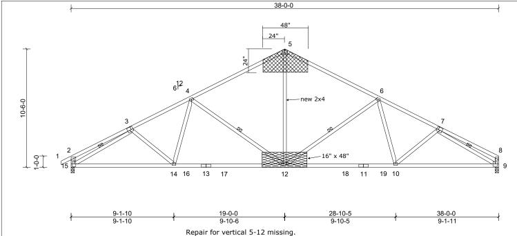
Cut and fit tight a new 2x4 SP or SPF No.2 vertical and attach 1/2" Plywood or 7/16" OSB (APA Rated Sheathing Exposure 1) gussets to both sides of truss as shown with two rows of 10d (.131" x 3") nails spaced 4" oc in all members from each face, driven through both sheets of plywood.
