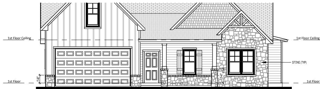
① Opt. Brick Skirt - Front Elevation 1/8" = 1'-0"
