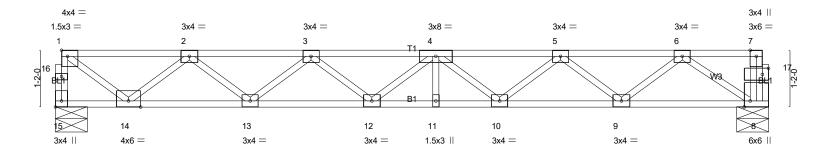
14-7-12 Plate Offsets (X,Y)-- [1:Edge,0-1-8], [8:0-1-8,Edge], [15:Edge,0-1-8], [17:0-1-8,0-1-8] LOADING (psf) SPACING-DEFL PLATES **GRIP** 2-0-0 CSI. in (loc) I/defl I/d **TCLL** 40.0 Plate Grip DOL 1.00 TC 0.29 Vert(LL) -0.1311 >999 480 MT20 244/190 TCDL 10.0 Lumber DOL 1.00 вс 0.51 Vert(CT) -0.18 >968 360 **BCLL** YES WB 0.51 0.04 0.0 Rep Stress Incr Horz(CT) 8 n/a n/a BCDL Code IRC2021/TPI2014 Matrix-SH Weight: 76 lb FT = 20%F, 11%E
