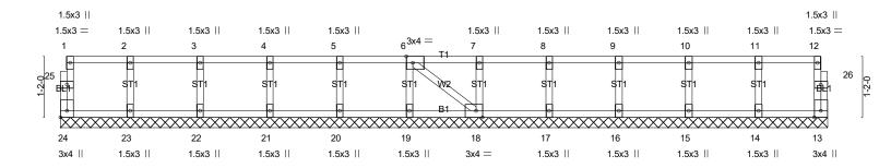
14-7-12 14-7-12 Plate Offsets (X,Y)-- [6:0-1-8,Edge], [18:0-1-8,Edge], [24:Edge,0-1-8] LOADING (psf) SPACING-CSI. DEFL. PLATES **GRIP** 2-0-0 in (loc) I/defl I/d **TCLL** 40.0 Plate Grip DOL 1.00 TC 0.06 Vert(LL) n/a n/a 999 MT20 244/190 TCDL 10.0 Lumber DOL 1.00 вс 0.01 Vert(CT) n/a n/a 999 **BCLL** YES WB 0.03 Horz(CT) 0.00 0.0 Rep Stress Incr 13 n/a n/a BCDL Code IRC2021/TPI2014 Matrix-SH Weight: 64 lb FT = 20%F, 11%E
