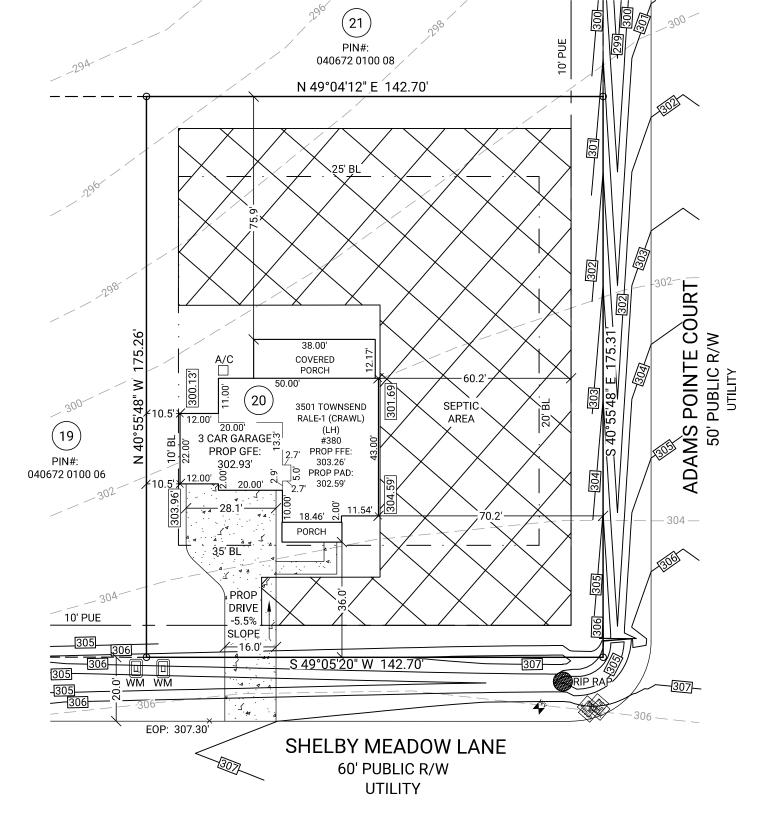
**LEGEND** BL**Building Line** Private Drainage Easement PDE **FFE** Finished Floor Elevation A/C Air Conditioning CI **Curb Inlet** R/W Right of Way Porch EΡ Electic Pedestal ΤP Telephone Pedestal Clean Out CO
