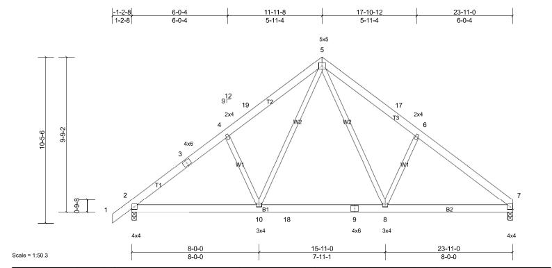
Plate Grip DOL TCLL (roof) Vert(LL) **TCDL** 10.0 Lumber DOL 1.15 BC 0.27 Vert(CT) -0.10 8-10 >999 240 **BCLL** 0.0\* Rep Stress Incr YES WB 0.39 Horz(CT) 0.02 7 n/a n/a BCDL IRC2021/TPI2014 Matrix-AS Wind(LL) Weight: 173 lb FT = 25% 10.0 Code 0.02 10 >999 240
