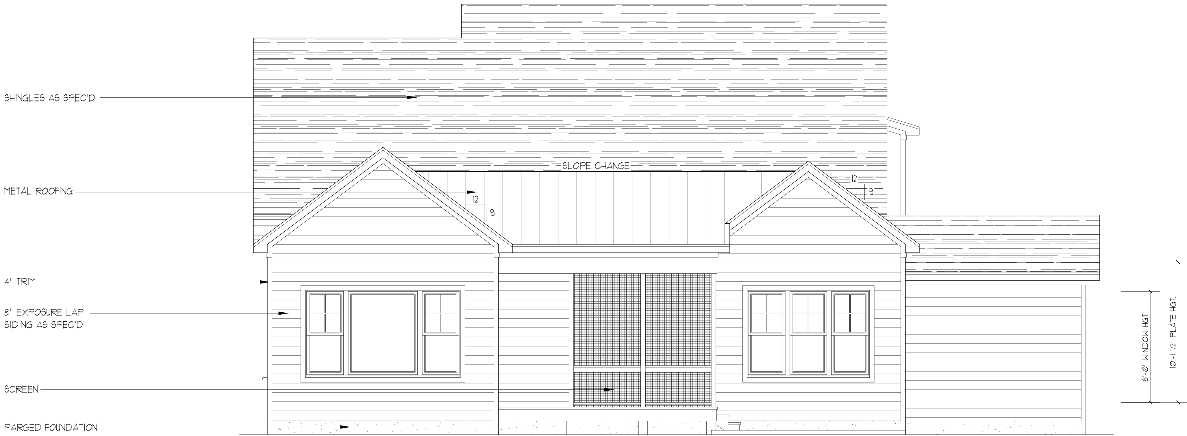
REAR ELEVATION SCALE: ----- 1/4" = 1'-0"
