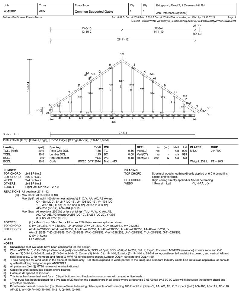
10) Beveled plate or shim required to provide full bearing surface with truss chord at joint(s) Q.
