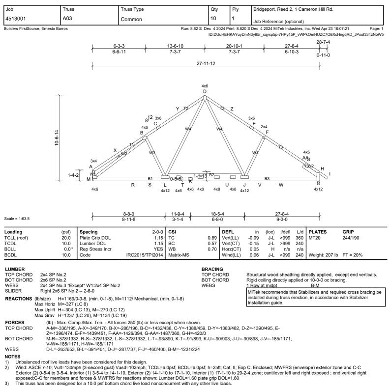
4) \* This truss has been designed for a live load of 20.0psf on the bottom chord in all areas where a rectangle 3-06-00 tall by 2-00-00 wide will fit between the bottom chord and any other members, with BCDL = 10.0psf.
