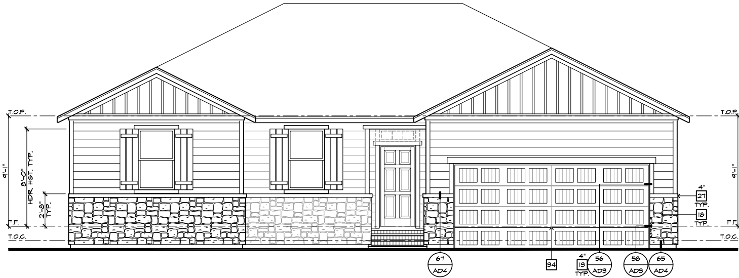
FRONT ELEVATION 'M' W/ STONE AT CRAWL SPACE AT OPTIONAL 9'-1" PLT. HGT. SCALE 1/4"=1'-0" (22"X34") - 1/8"=1'-0" (11"X17")
