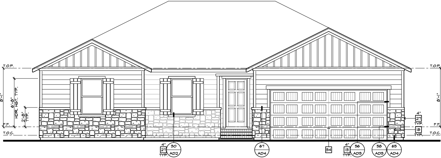
FRONT ELEVATION 'M' W/ STONE AT CRAWL SPACE SCALE 1/4"=1'-0" (22'X34") - 1/8"=1'-0" (11'X17")
