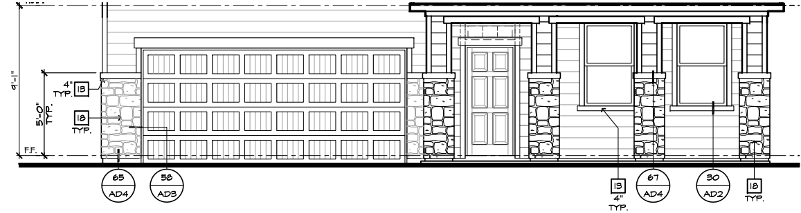
PARTIAL FRONT ELEVATION 'N' AT OPTIONAL 9'-1" PLT. HGT. W/ STONE OPT. SCALE 1/4"=1'-0" (22'X34') - 1/8"=1'-0" (11'X17')
