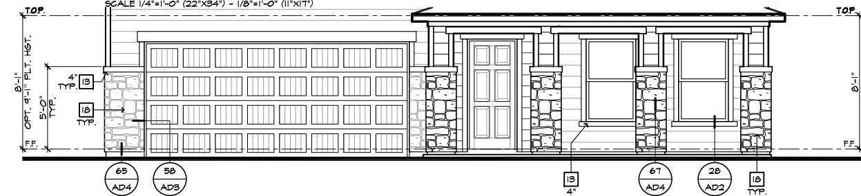
PARTIAL FRONT ELEVATION 'N' W/ STONE OPTION SCALE 1/4"=1'-0" (22"X34") - 1/8"=1'-0" (11"X17")
