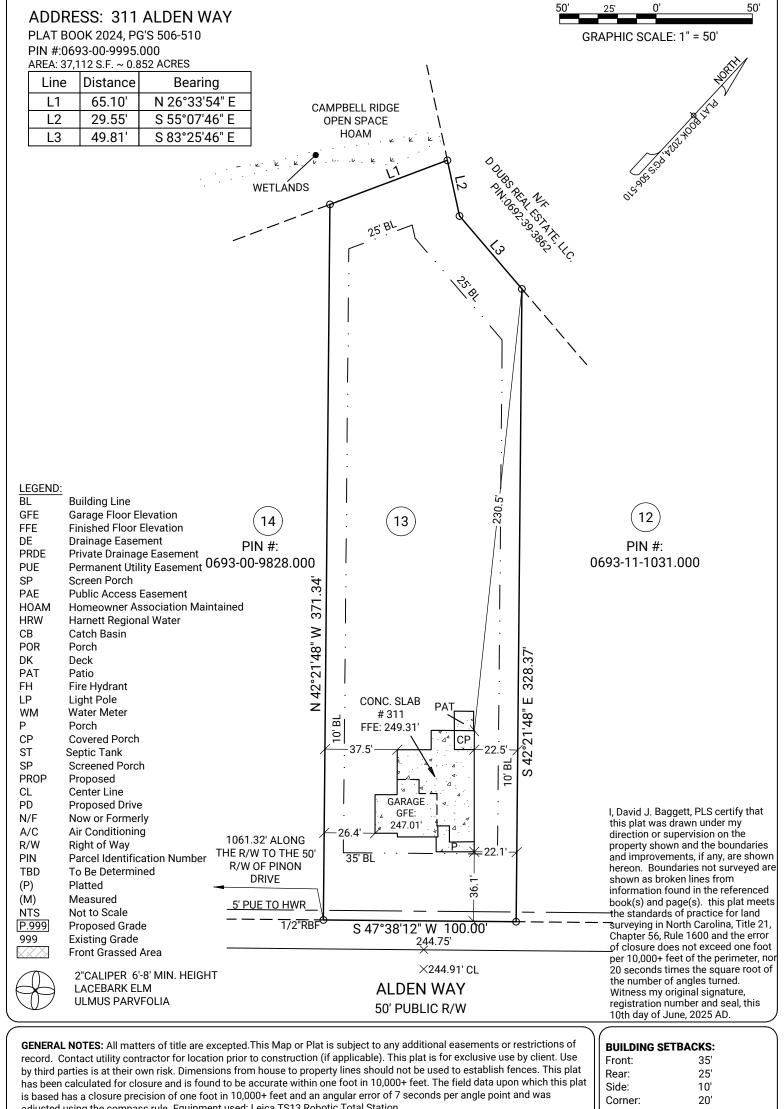
adjusted using the compass rule. Equipment used: Leica TS13 Robotic Total Station.
