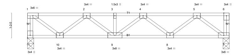
Plate Offsets (X,Y)-- [11:Edge,0-1-8] LOADING (psf) SPACING-2-0-0 CSI. DEFL. I/defl L/d **PLATES GRIP** (loc) TCLL Ÿ0.Ó Plate Grip DOL 1.00 TC 0.32 Vert(LL) -0.02 ģ >999 480 MT20 244/190 **TCDL** 10.0 Lumber DOL 1.00 ВС 0.24 Vert(CT) -0.03 8-9 >999 360 **BCLL** 0.0 Rep Stress Incr NO WB 0.31 Horz(CT) 0.01 n/a n/a **BCDL** 5.0 Code IRC2021/TPI2014 Matrix-SH Weight: 51 lb FT = 20%F, 11%E
