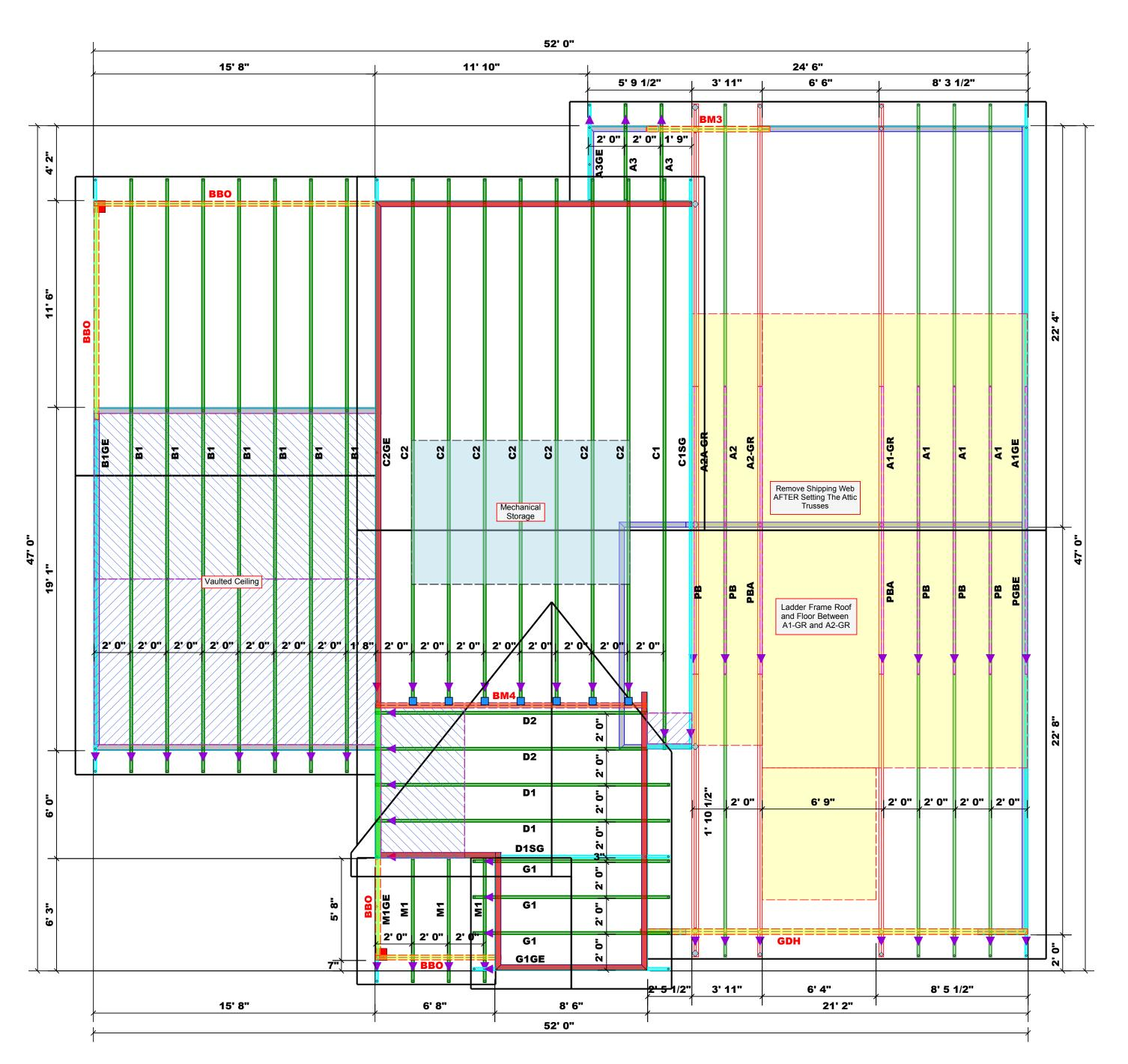
Dimension Notes All exterior wall to wall dimensions are to face of sheathing unless noted otherwise 2. All interior wall dimensions are to face of frame wall unless noted otherwise 3. All exterior wall to truss dimensions are to face of frame wall unless noted otherwise
