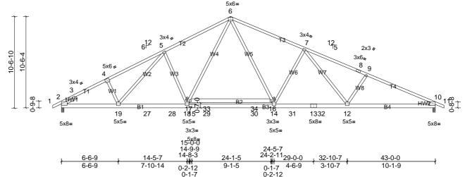
Plate Offsets (X, Y): [2:Edge,0-2-1], [4:0-3-0,0-3-0], [10:Edge,0-1-6] CSI DEFL 2-0-0 in I/defl L/d **PLATES** Loading (psf) Spacing (loc) TCLL (roof) 20.0 Plate Grip DOL 1.15 TC 0.97 Vert(LL) -0.36 16-17 >999 240 MT20
