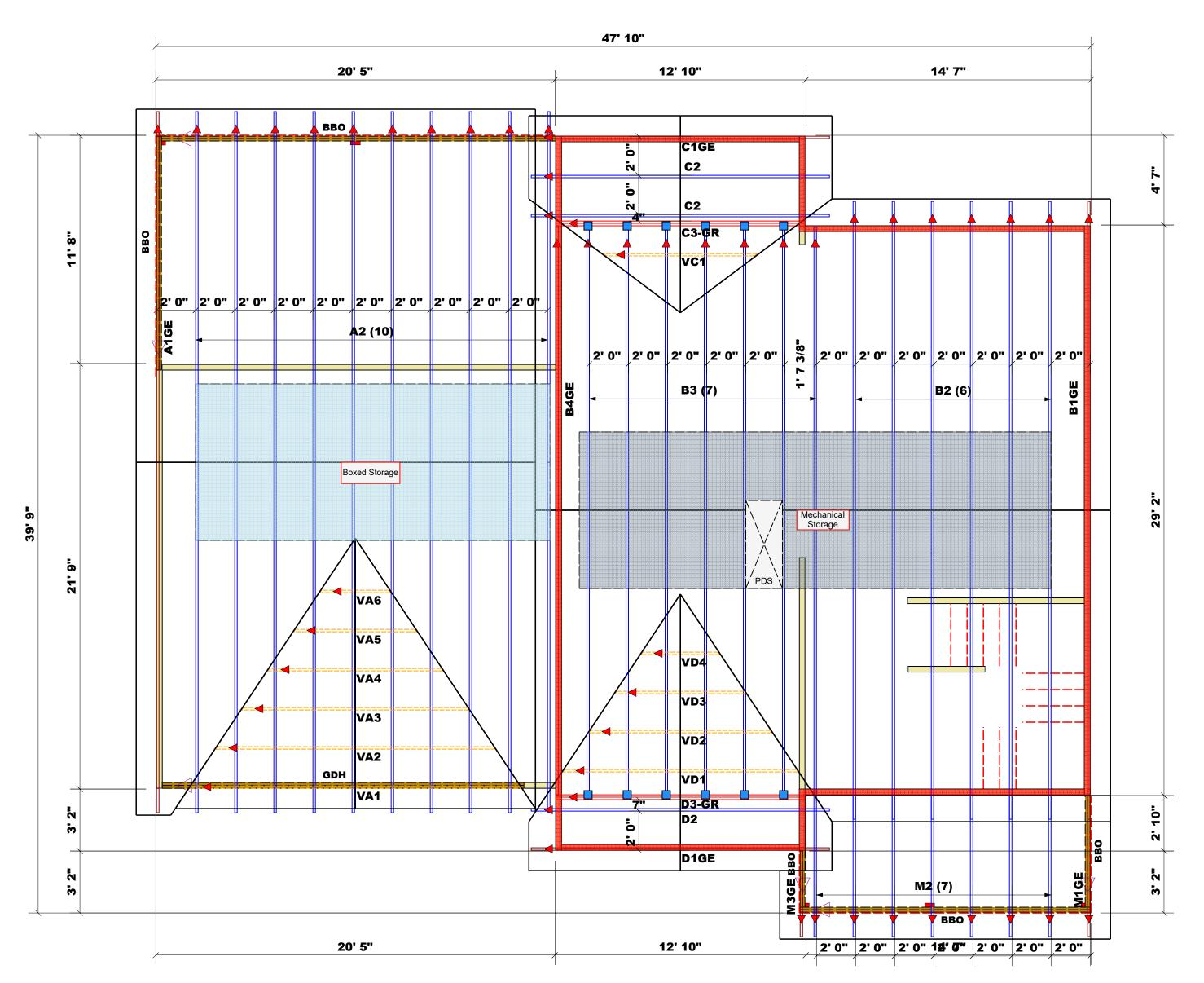
Plumbing Drop Notes 1. Plumbing drop locations shown are NOT exact. 2. Contractor to verify ALL plumbing drop locations prior to setting Floor Trusses. 3. Adjust spacing as needed not to exceed 24"oc
