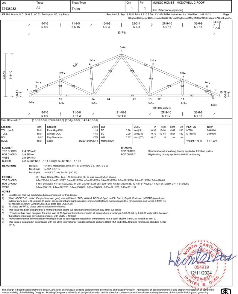
codes and ordinances. Building Designer accepts responsibility for the correctness or accuracy of the design information as it may relate to a specific building. Certification is valid only when truss is fabricated by a UFPI plant. Bracing shown is for lateral support of truss members only and does not replace erection and permanent bracing. Refer to Building Component Safety Information (BCSI)
