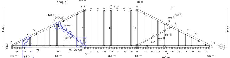
ATTACH 1/2" PLYWOOD OR OSB GUSSET (15/32" RATED SHEATHING 32/16 EXP 1) TO ONE FACE OF TRUSS WITH (0.113" X 2") NAILS PER THE FOLLOWING NAIL SCHEDULE: 2 X 3'S - 2 ROWS, 2 X 4'S - 3 ROWS, 2 X 6'S AND LARGER - 4 ROWS: SPACED @ 2" O.C. INTO EACH COVERED TRUSS MEMBER. USE 2" MEMBER END DISTANCE.
