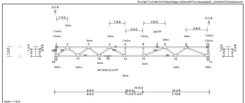
Plate Offsets (X, Y): [13:0-1-8,Edge], [14:0-1-8,Edge], [18:0-2-0,Edge]
