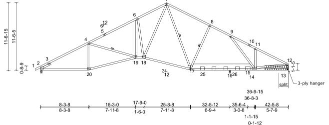
Repair for 2" high x 16" long section split from the bottom chord at joint 13.
