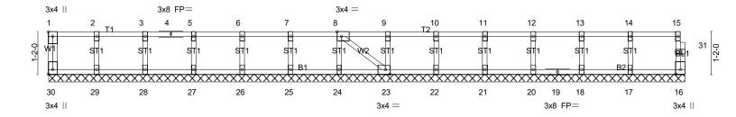
Plate Offsets (X,Y)-- [1:Edge,0-1-8], [8:0-1-8,Edge], [23:0-1-8,Edge], [30:Edge,0-1-8] LOADING (psf) SPACING-2-0-0 CSI. DEFL. I/defl L/d **PLATES GRIP** in (loc) TC BC TCLL Ÿ0.Ó Plate Grip DOL 1.00 0.07 Vert(LL) 999 MT20 244/190 n/a n/a **TCDL** 10.0 Lumber DOL 1.00 0.01 Vert(CT) n/a n/a 999 **BCLL** 0.0 Rep Stress Incr YES WB 0.03 Horz(CT) 0.00 16 n/a n/a **BCDL** 5.0 Code IRC2021/TPI2014 Matrix-SH Weight: 76 lb FT = 20%F, 11%E
