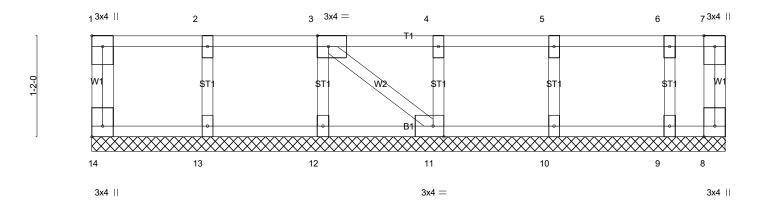
Plate Offsets (X,Y)-- [1:Edge,0-1-8], [3:0-1-8,Edge], [11:0-1-8,Edge], [14:Edge,0-1-8] LOADING (psf) SPACING-2-0-0 CSI. DEFL. I/defl L/d **PLATES GRIP** in TC BC TCLL Ÿ0.Ó Plate Grip DOL 1.00 0.06 Vert(LL) 999 MT20 244/190 n/a n/a **TCDL** 10.0 Lumber DOL 1.00 0.01 Vert(CT) n/a n/a 999 **BCLL** 0.0 Rep Stress Incr YES WB 0.03 Horz(CT) 0.00 11 n/a n/a **BCDL** 5.0 Code IRC2021/TPI2014 Matrix-P Weight: 36 lb FT = 20%F, 11%E
