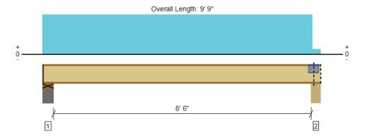
Member Length : 9' 7 7/8" System : Floor Member Type : Joist Building Use : Residential Building Code : IBC 2021
