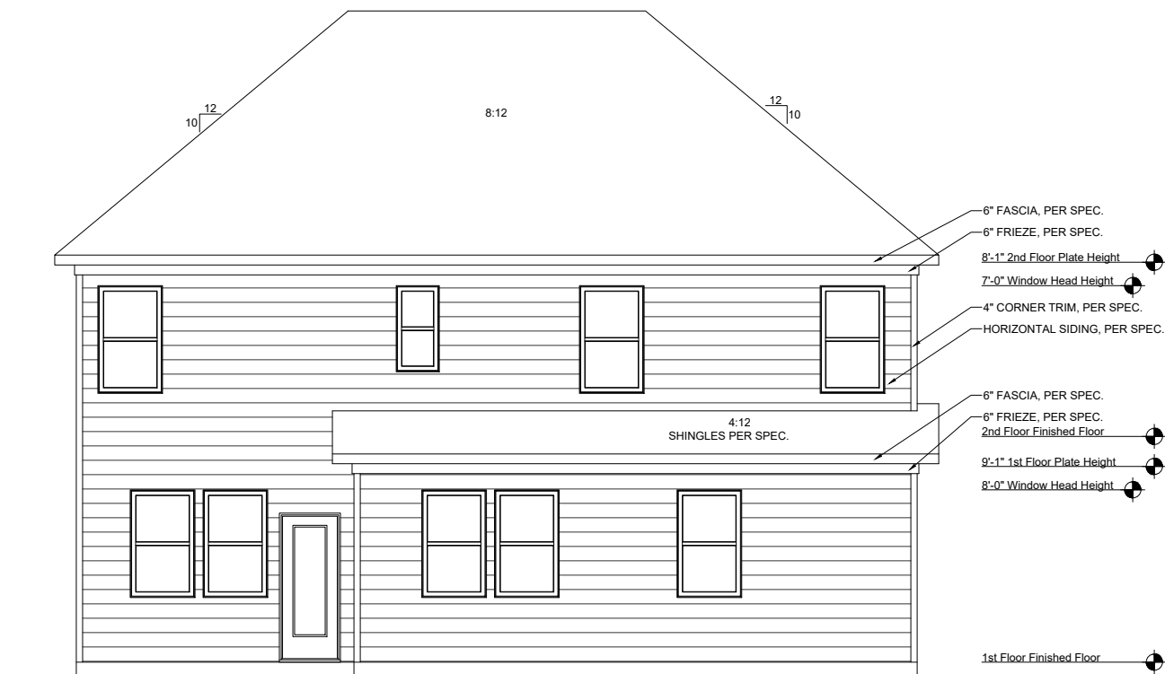
OPT. EXTENDED FAMILY REAR ELEVATION SCALE: 1/8"=1'-0" (11"X17" SHEET SIZE) SCALE: 1/4"=1'-0" (22"X34" SHEET SIZE)
