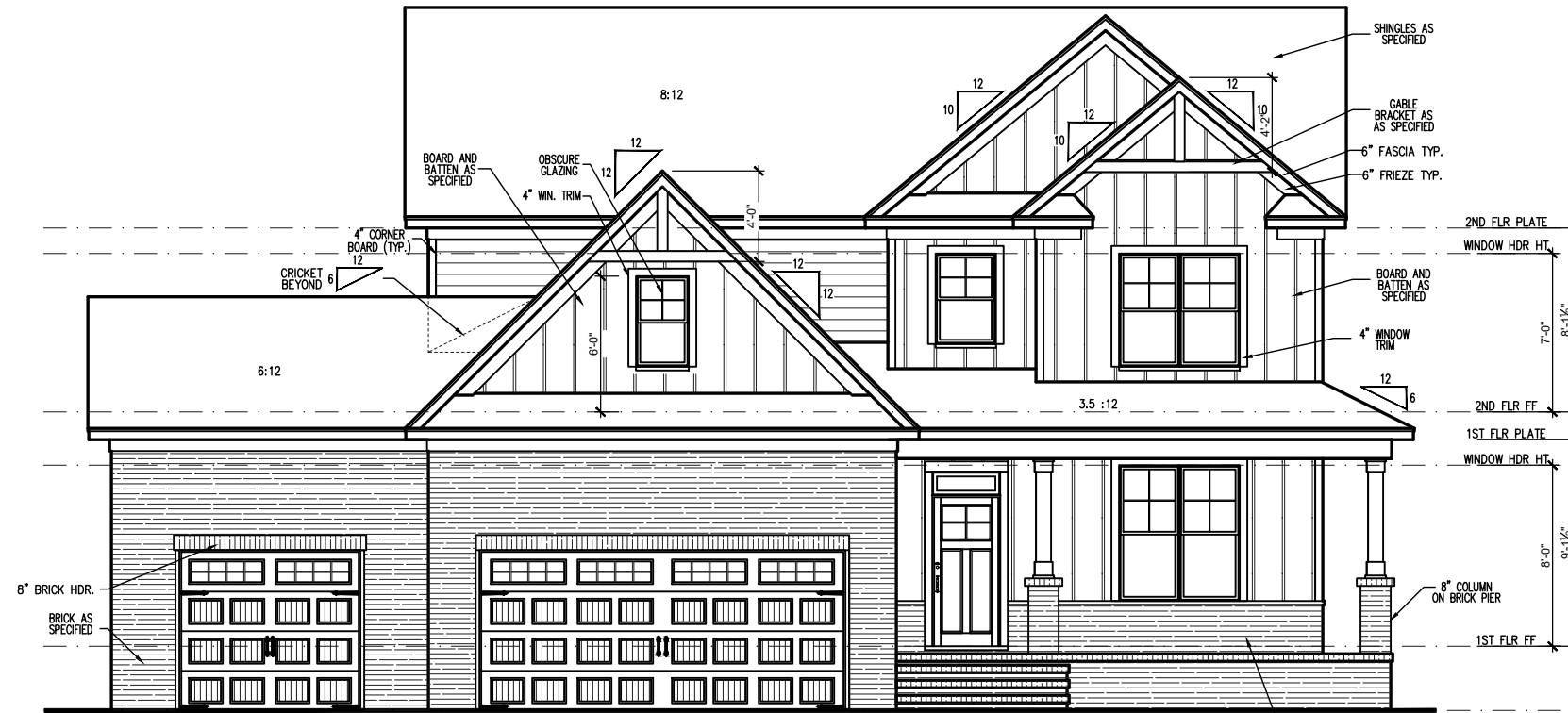
FRONT ELEVATION 'E' - 3 CAR FRONT LOAD (CRAWL)
